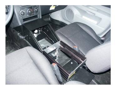
View of installed C-VS-0812-CHGR
